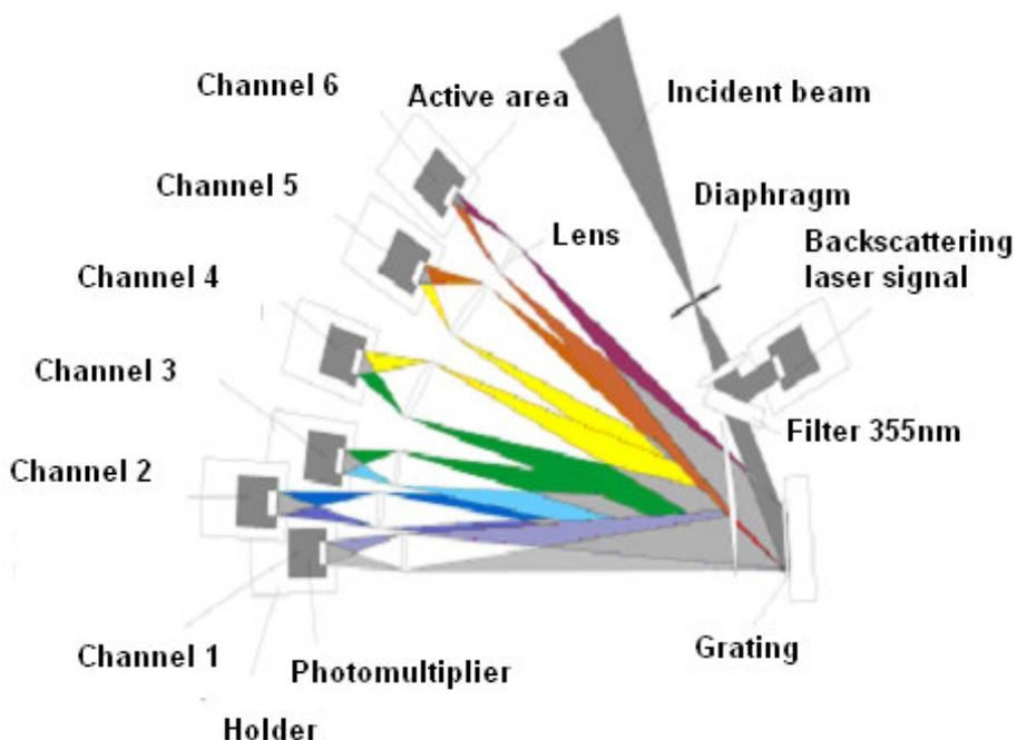
Figure 1: Optical design of the polychromator
