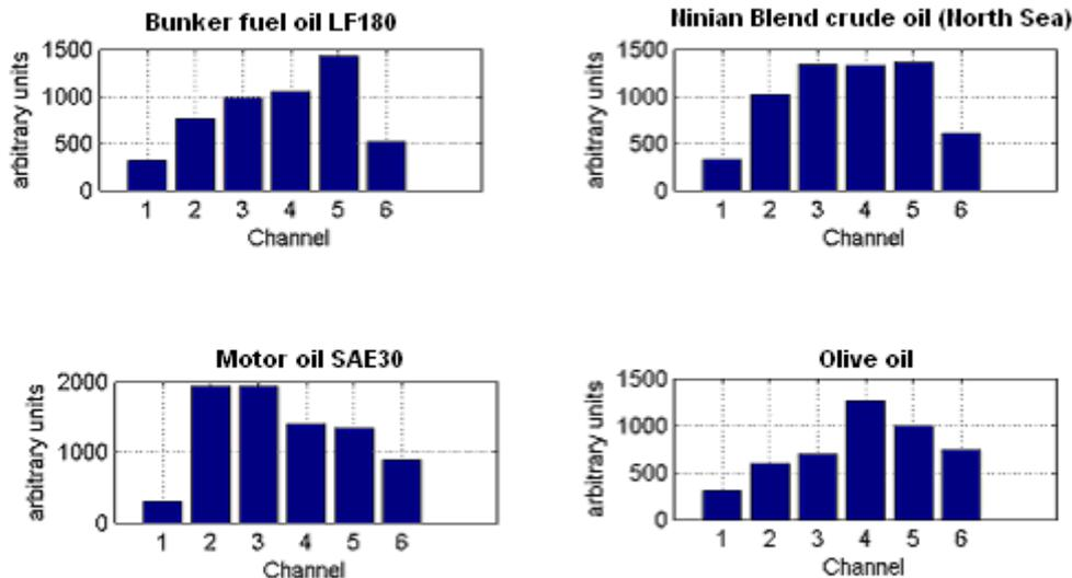
Figure 2: Examples of oil spectra spectrally grouped according to the detection channel wavebands of the laser fluorosensor.
